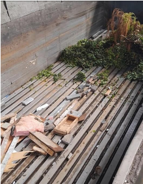
Figure 10.2: Walking floor with material disposed of as general waste containing building material and green waste.
