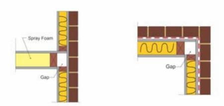
☐ Insulate closed corner external wall junctions before installing building wrap installation with conventional bats or fire retardant expanding foam.
