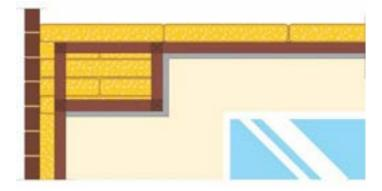
☐ For bathtubs on the outside walls, insulate the exterior wall and air-seal behind the bathtub with cement sheet or blue board (plywood, plaster, rigid foam insulation) before the tub is put into place. After the drain is installed, seal the tub drain penetration with caulk or spray foam.
