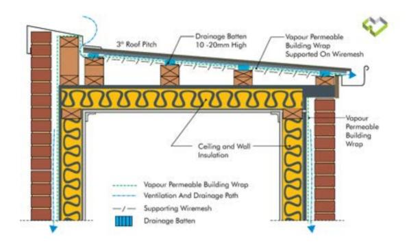
To further promote ventilation of the roof surface, drainage battens that allow air to pass through along the slope of the roof may be used. The air flow promotes drying and cooling. A batten 10 - 20mm high located between the roof building wrap and roof deck, will help provide a clear ventilation and drainage path.
