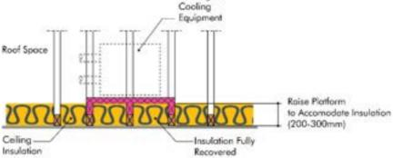
Mechanical Platforms must be raised to accommodate the full height of the ceiling insulation. To maintain the continuous performance of the ceiling insulation, the plant and equipment platform located in the ceiling/roof cavity must be raised to the depth of the selected insulation. Additional framing will be required, and insulation must be installed prior to plasterboard ceiling installation.
