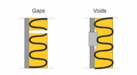
☐ Insulation must be installed with no gaps or voids on all surface areas of the building envelope including walls and ceilings to outside and junction points where the ceiling roof and walls are close together.
