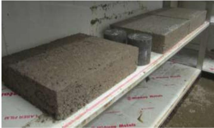
**Figure 16. Compacted slabs in fog room**
