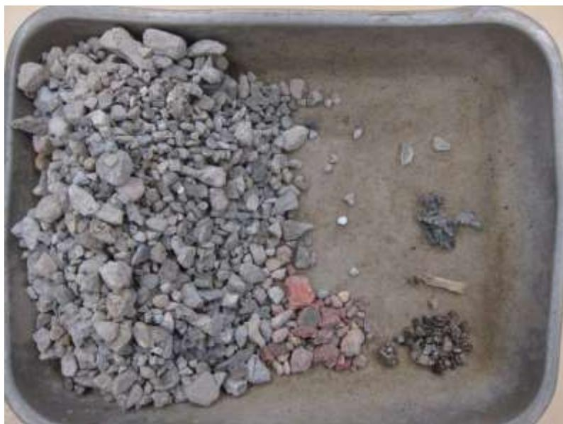
**Figure 1. Foreign material contents in crushed concrete**
